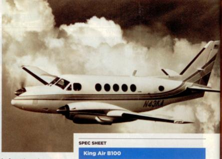
Engines | Two Honeywell TPE331-6-252B engines at 715 shaft horsepower each Seats | one or two pilots and six-10 passengers Max takeoff weight | 11,800 lbs Max cruise speed | 265 kts Takeoff distance | 1,898 ft Landing distance | 1,290 ft Range | 1,120 nm Wingspan | 45 ft, 11 in Length | 39 ft, 11 in Height | 15 ft, 5 in
